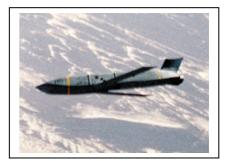
Performance: Power Plant = Teledyne CAE J402-CA-100 turbojet; 3.0 kN (680 lb) Accuracy = 3m Range = 205nm Speed = Subsonic glide weapon
