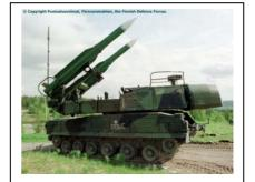
The SA-11 GADFLY is a medium-range, semi-active, radar-guided missile using solid-rocket propulsion that provides defense against high-performance aircraft and cruise missiles. The SA-N-7 GADFLY is the naval Version of the SA-11.
